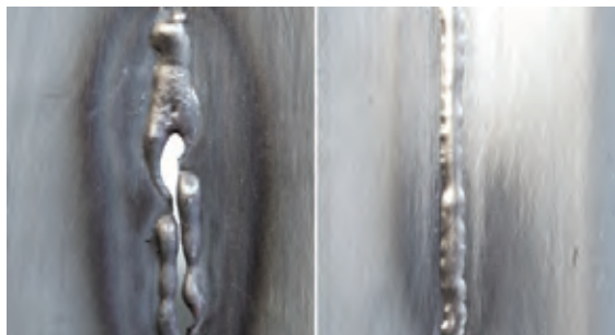
Ideal for sectional repairs with MIG-weld-seams
