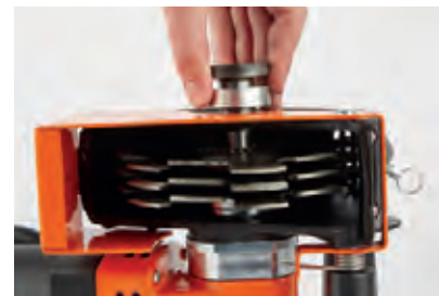
Effortless tool change thanks to split safety spindle and precision-fit spacer rings
