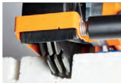
The small gap between the protective cover and the diamond cutting disc allows working as close as 18 mm to the edge.
