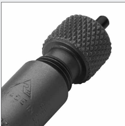
Knurled screw to widen the centring sleeve
