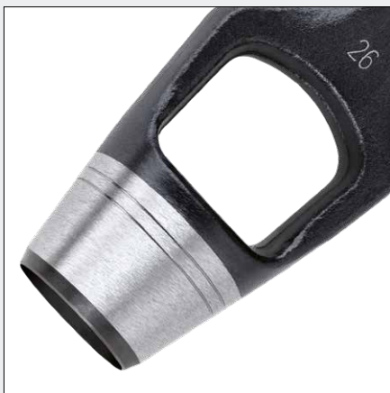
Conical cutting head, polished and blank, slightly conical on the inside to remove stamped out material
