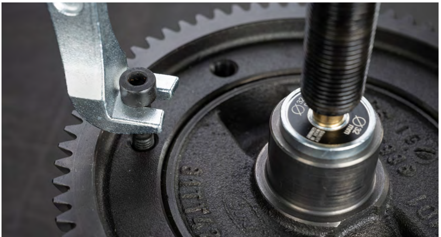
Extraction process of a camshaft gear with the 118-0 using the single-finger claws.
