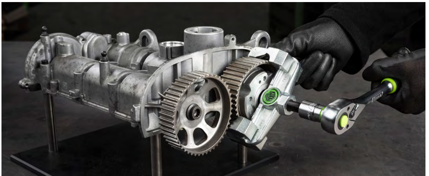
Both photos show the extraction process of a camshaft gear with the 118-0 using the single-finger claws.
