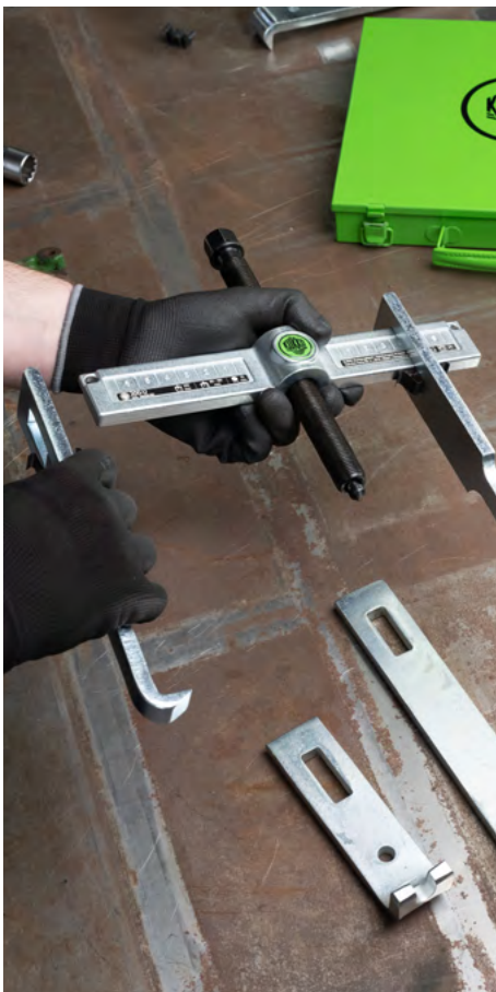
The puller jaws are placed on the crossbar; a scale on the crossbar facilitates the correct adjustment of the distances.
