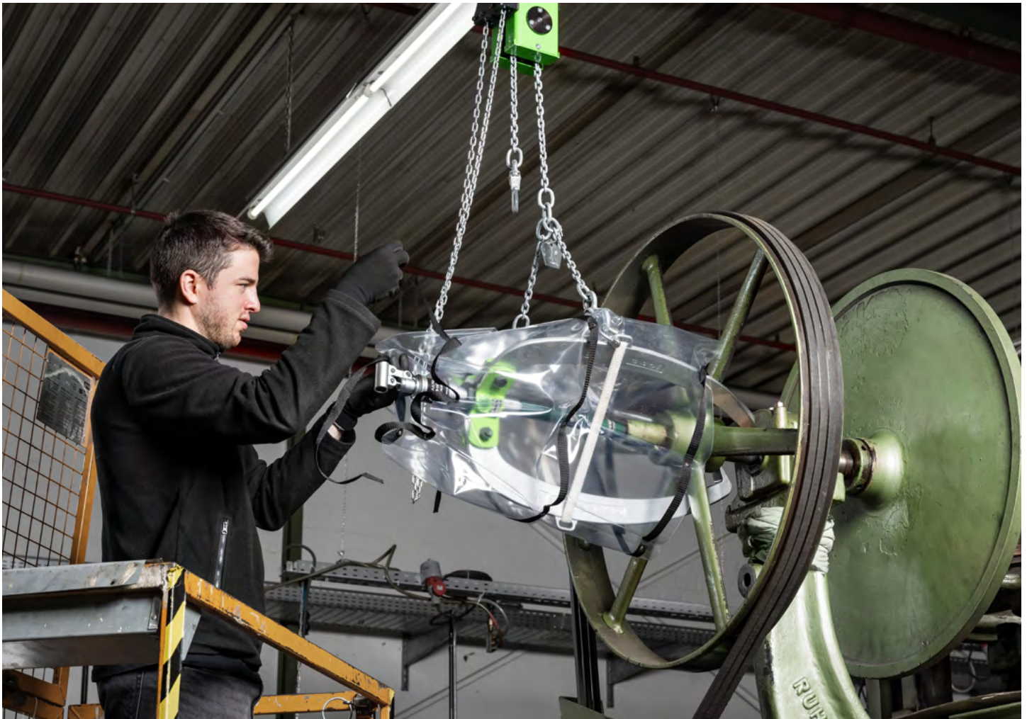
The UFP accident protection tarpaulin offers safety when removing a pulley from a press
