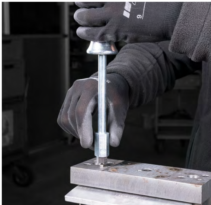
Removing a ball bearing using a sliding hammer, connecting nut and thread adapter
