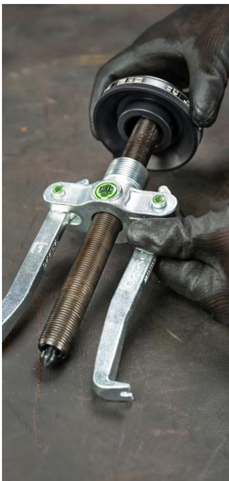
Mounting the clamping cone rotated by 180°
