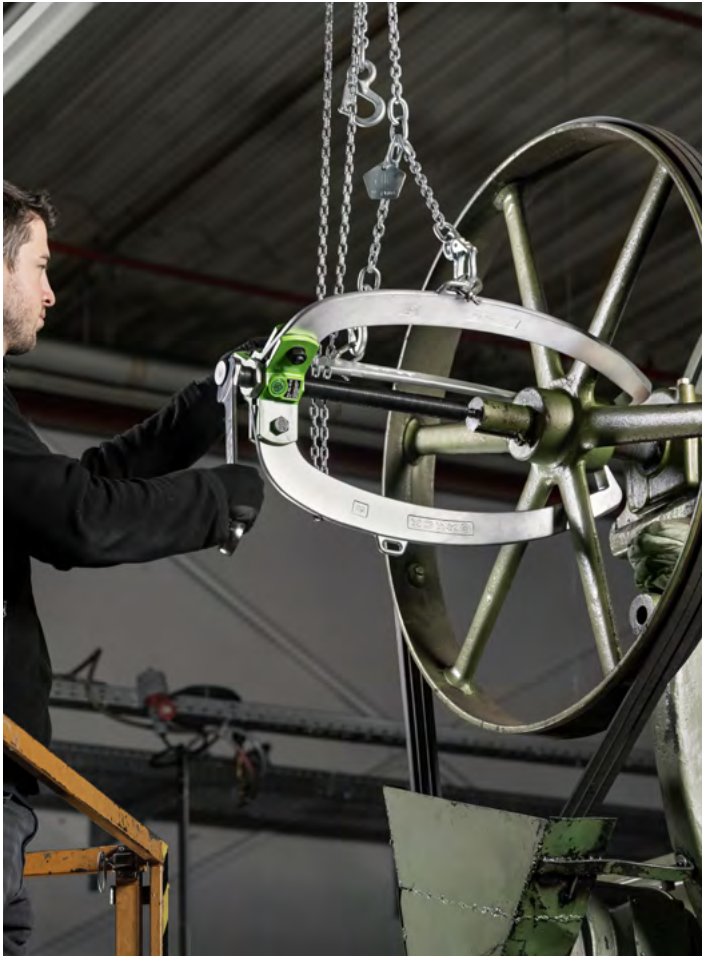
Removing a pulley with the 45-8 using a mechanical spindle. The puller is connected to the URANUS for locking and holding.
