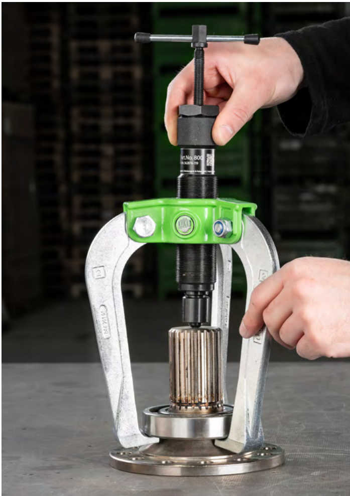
Tensioning the puller by screwing in the hydraulic spindle at the knurling.
