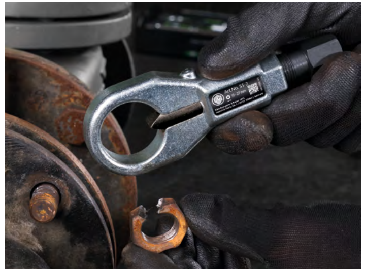
After the explosive release, the mother can be easily removed from the thread.
