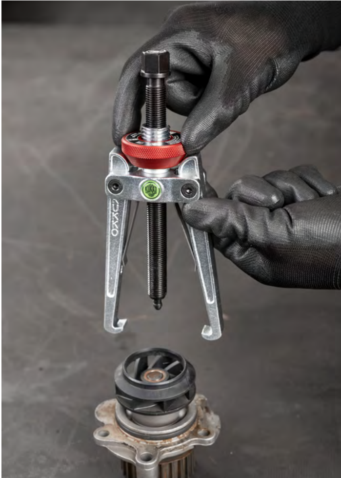
The 2-jaw puller 112-20 with cone knob during the extraction of a ball bearing on a water pump
