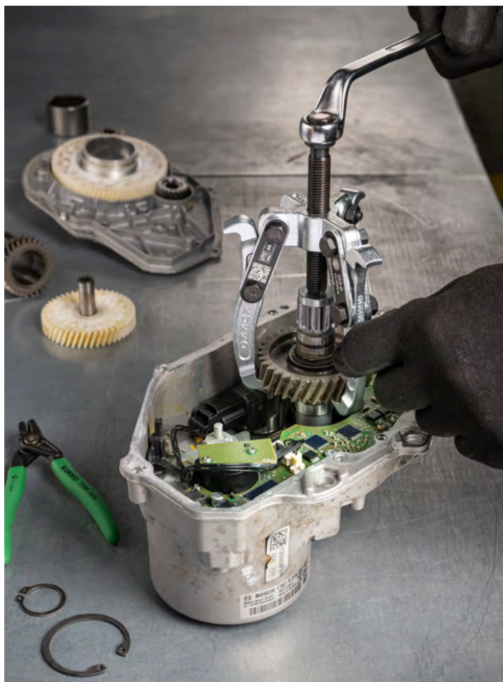
3-jaw puller with combination crossbar for the removal of a gear from an electric motor
