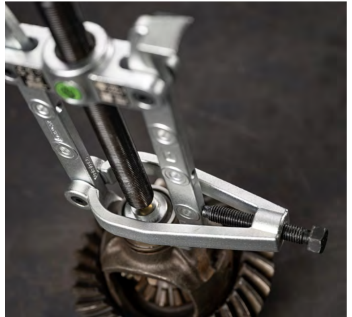
The clamp firmly presses the puller jaws against the part to be removed.
