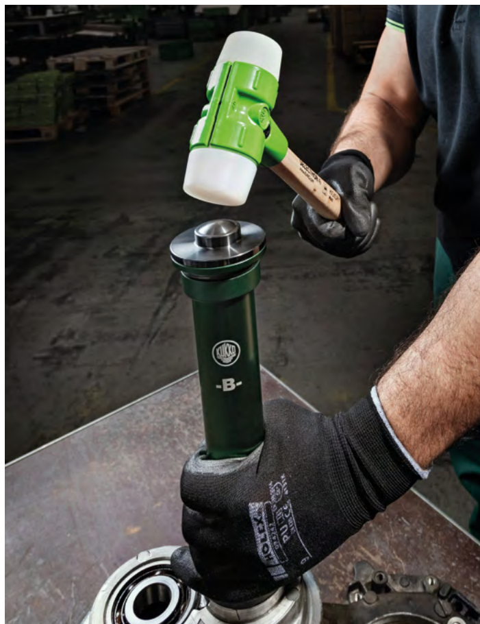
Installation of a bearing with a soft-face hammer Selector in combination with the 71-L
