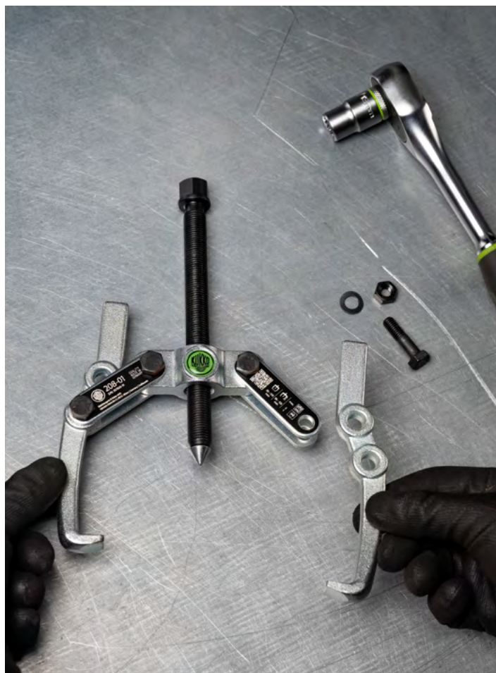
Conversion for adjusting the reach depth and span using the example of the 208-01.
