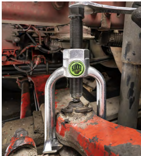
The ball joint puller 128-60 when pressing a steering track end on a tie rod in a workshop
