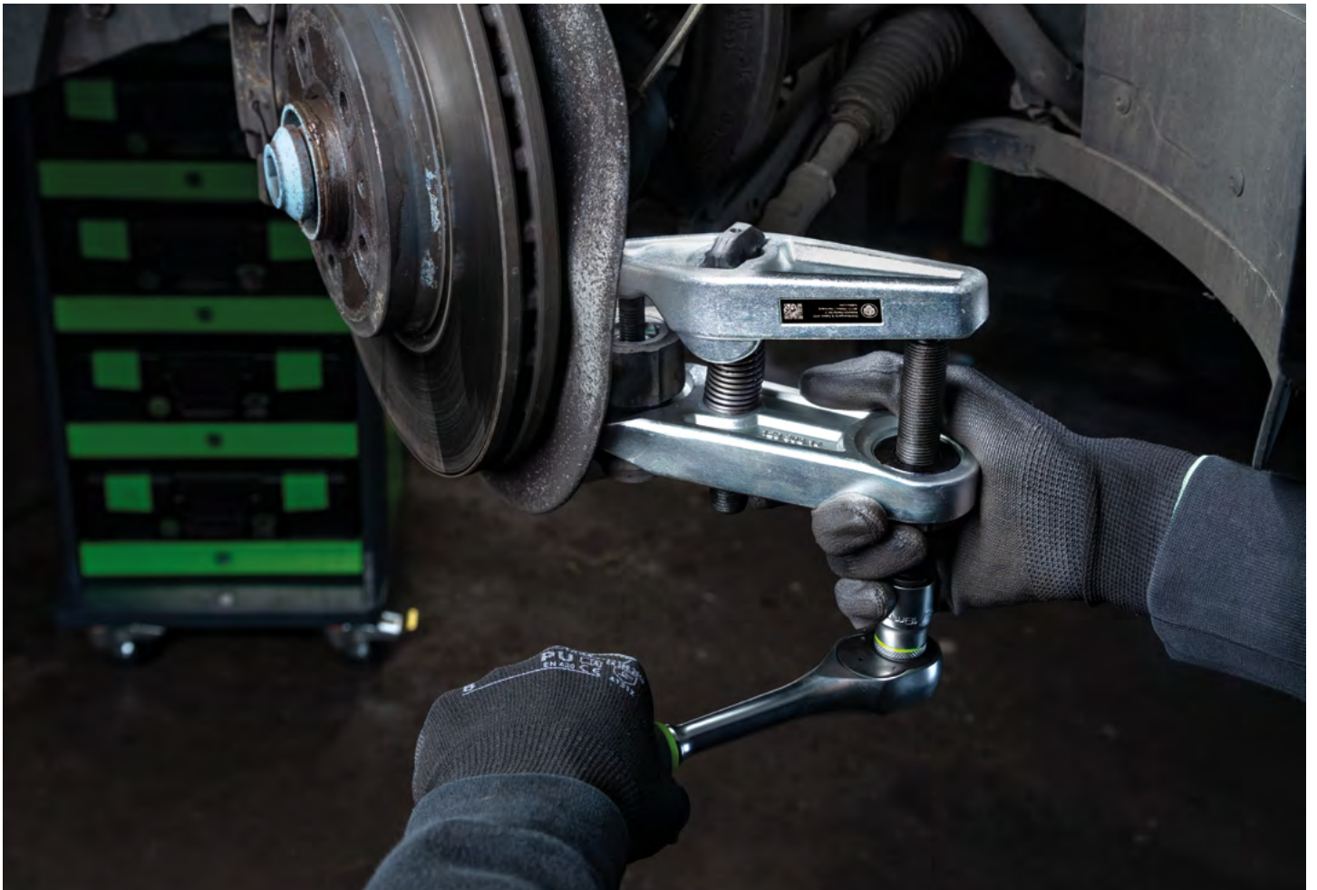
The ball joint extractor 129-3 when pressing out a track rod knob
