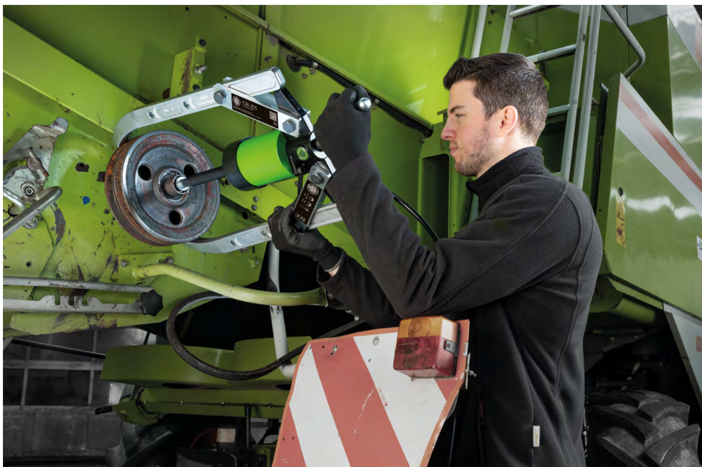
External extraction of a pulley on a combine harvester with the hydraulic puller Y28-205
