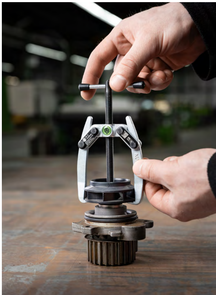
Removing a pump wheel from a water pump on the car with the 41-2
