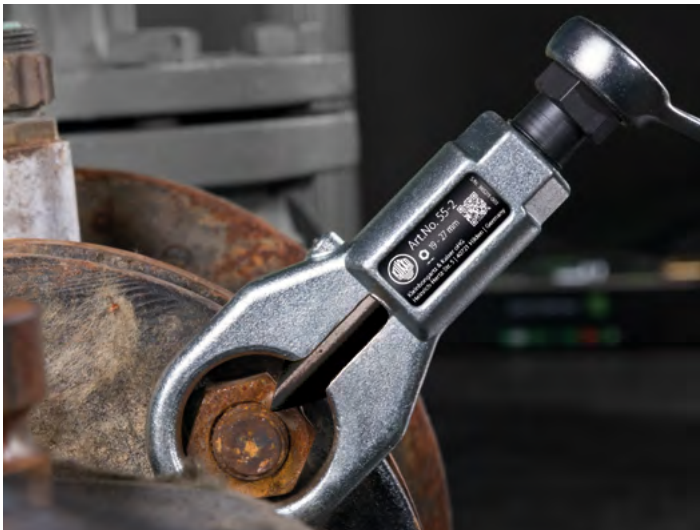
By pulling the spindle, the chisel is pressed into the nut to be split.
