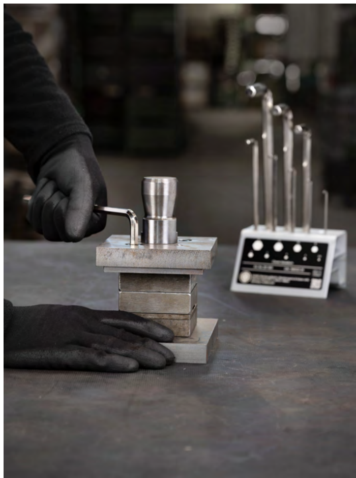
The angle screwdrivers from the sales and workshop stand ISO 2936 during the disassembly of a stamping tool.
