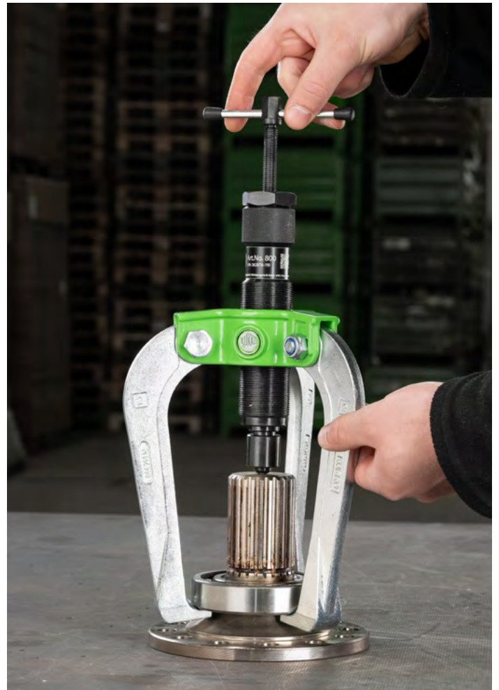
Actuation of the T-handle for the construction of hydraulic power
