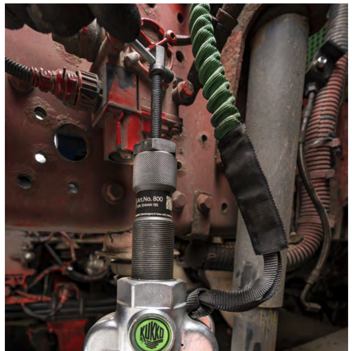
Safety puller secures ball joint puller
