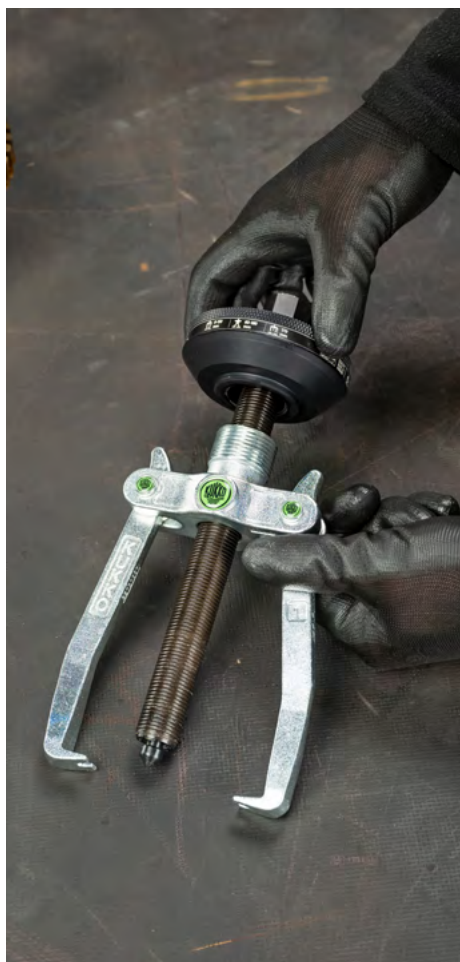
Removing the clamping cone
