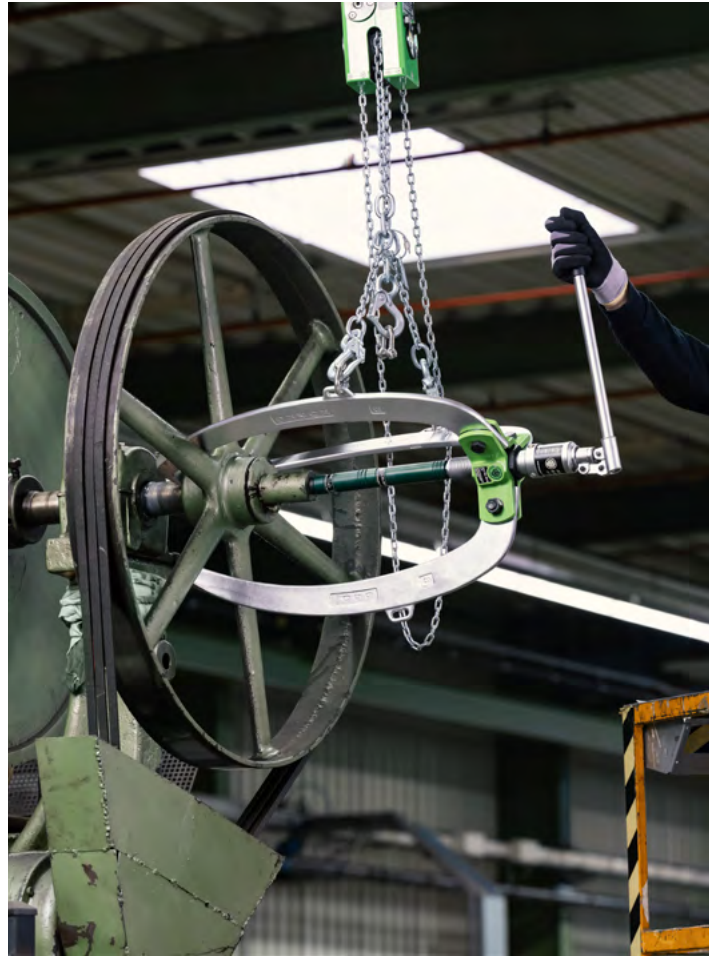
Removing a pulley with the 45-8 with hydraulic spindle
