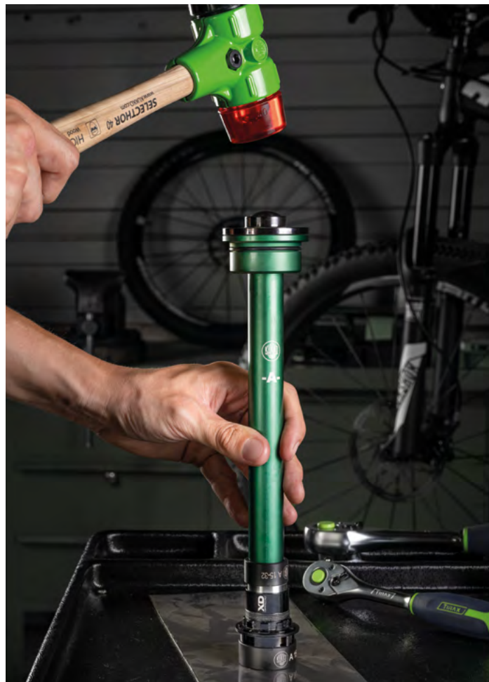
Pressing a bearing using a K-71
