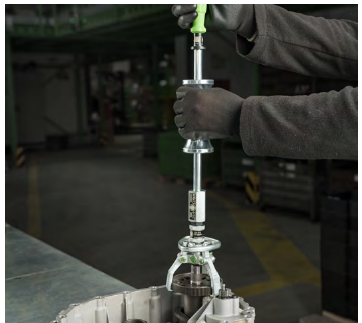
Dismantling a pulley from a transmission part
