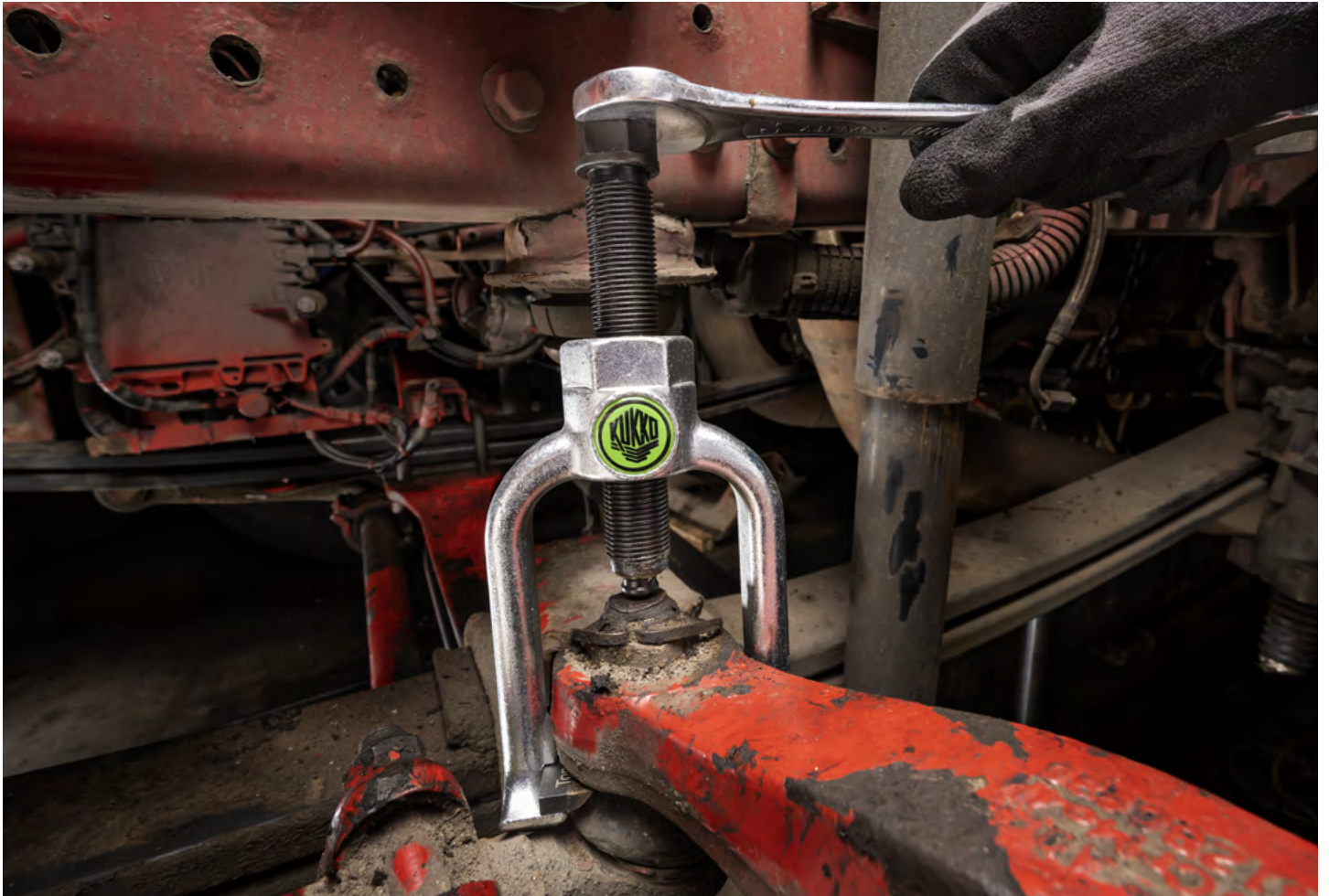
The ball joint puller 128-60 when pressing out a tie rod end on a track rod
