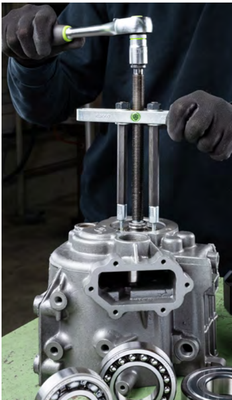
Ball bearing disassembly with the 69-A
