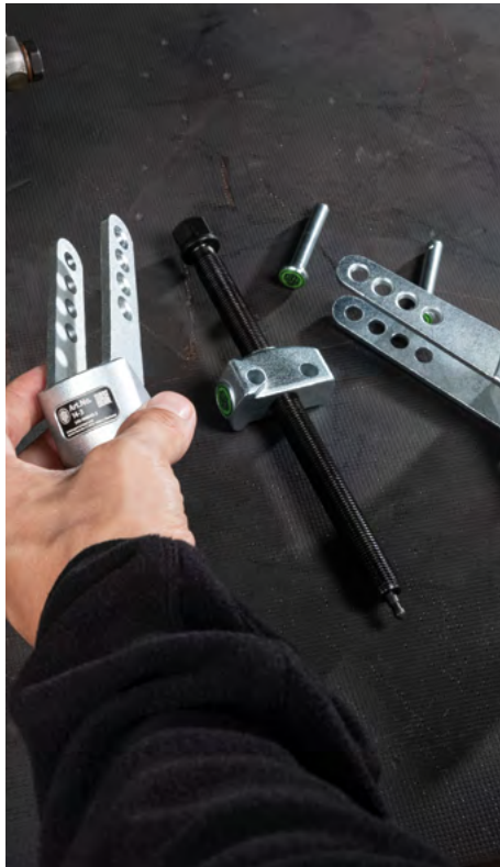
New combining of the individual components and reversing the jaws
