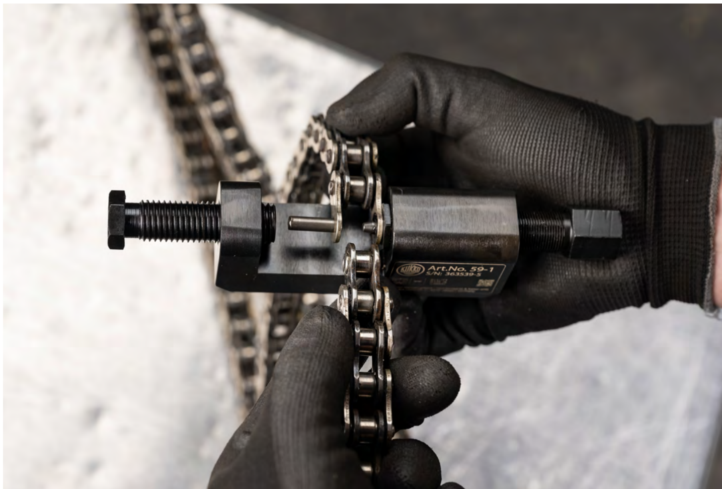
The bolt of a chain was pressed out with the chain breaker 59-1
