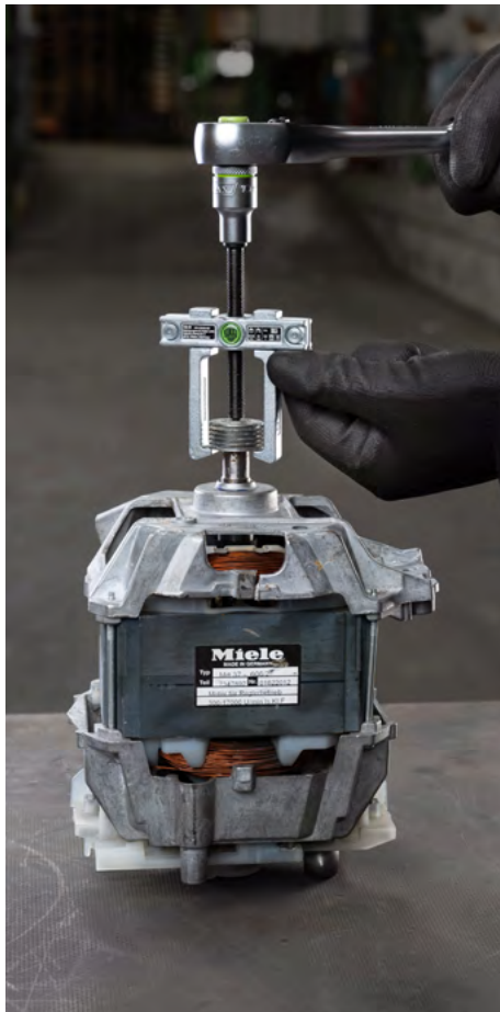
Removing a pulley from a washing machine motor with the 110-01
