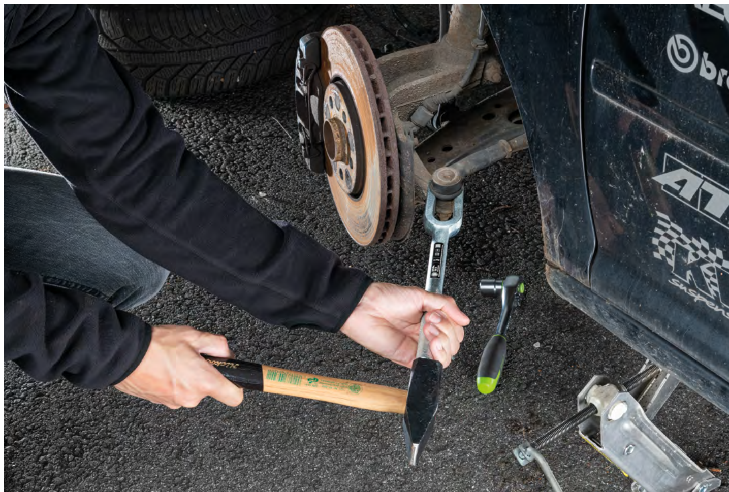
The separating fork 135-2 when releasing a ball joint wedged into the cone seat of a car
