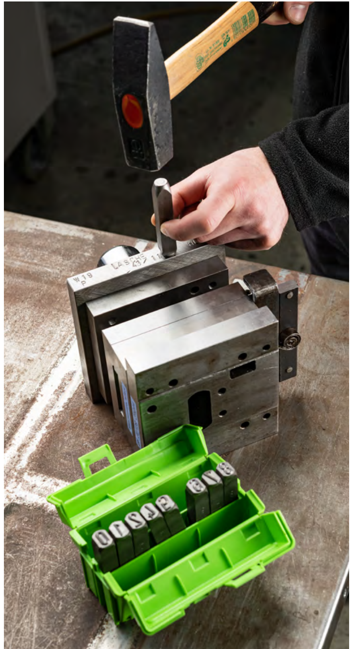
Marking a punching tool with impact numbers of series 328
