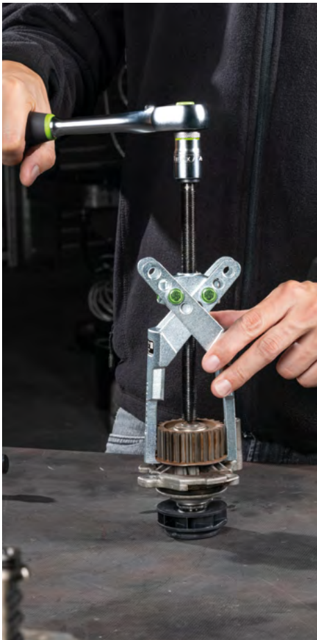
The scissor-like hook guide ensures a secure hold. The claws encompass the pulley.
