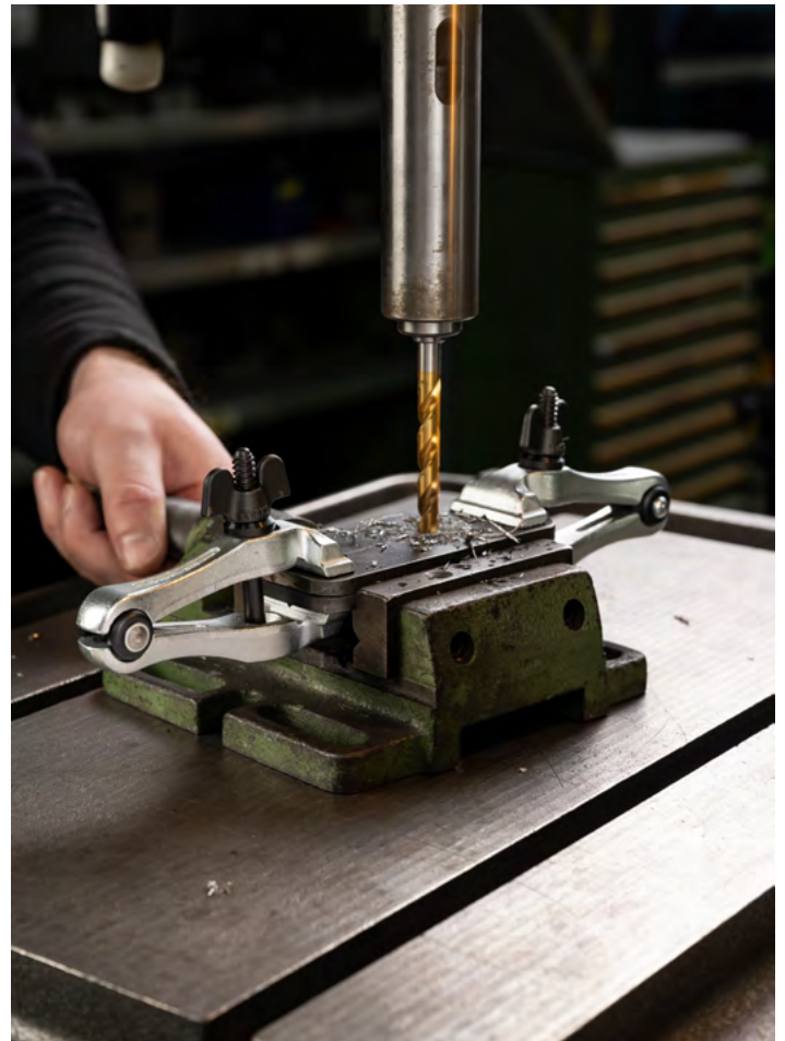
Two hand vises 101-100 for clamping several workpieces for drilling operations.
