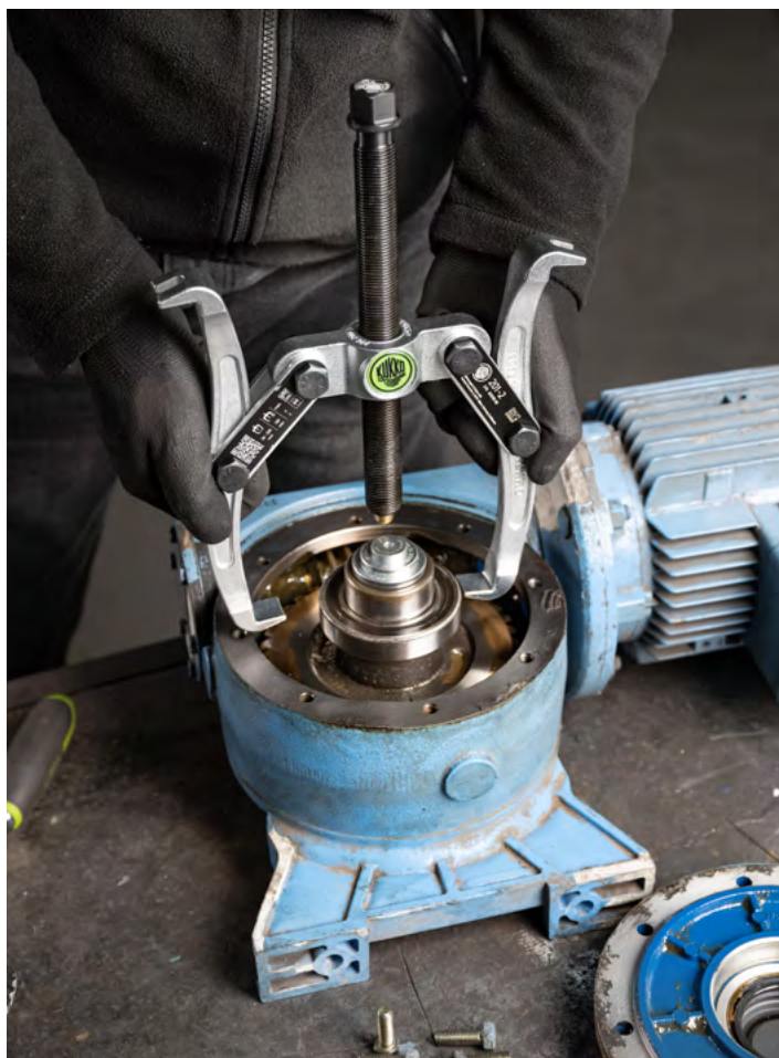
The oscillating jaws of the series 201, 202, and 203 can be perfectly positioned on the part to be pulled out.
