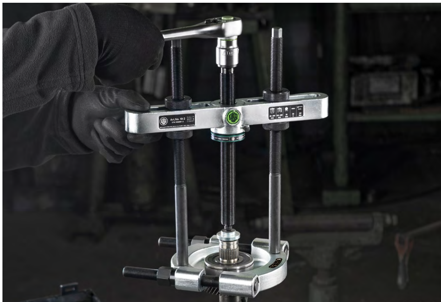
The separating device 15-2 during the removal of a fixed gear wheel on a machine component
