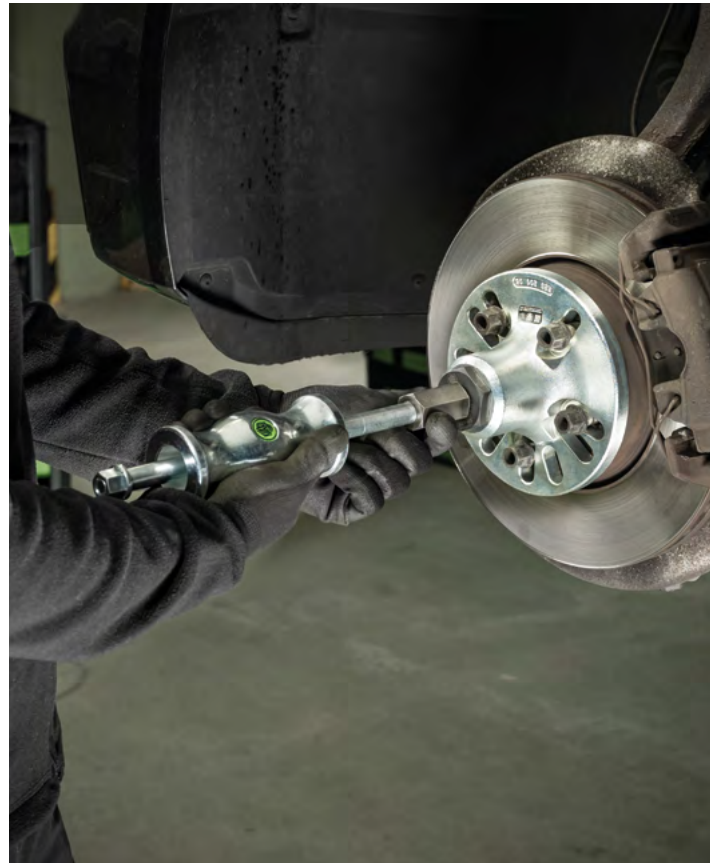
The hub puller 229-1-1 with sliding hammer for extracting stuck wheel hubs on a passenger car.
