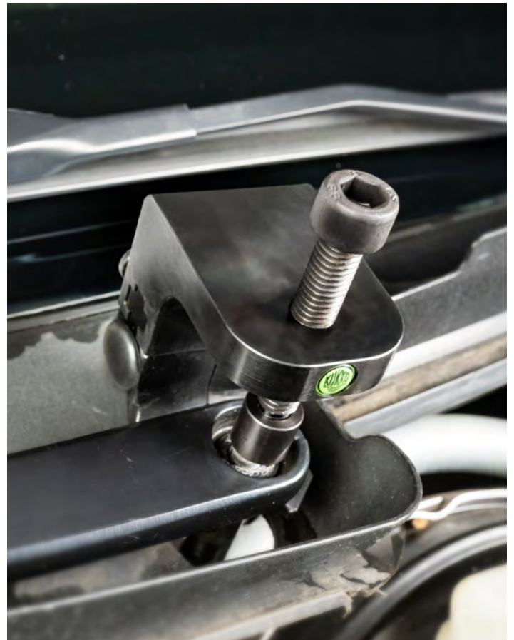
Removing a wiper arm with the 128-F-60
