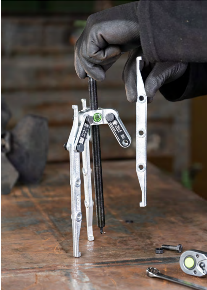
The multi-drilling in the puller jaws guarantees an individual adjustment to the reach.
