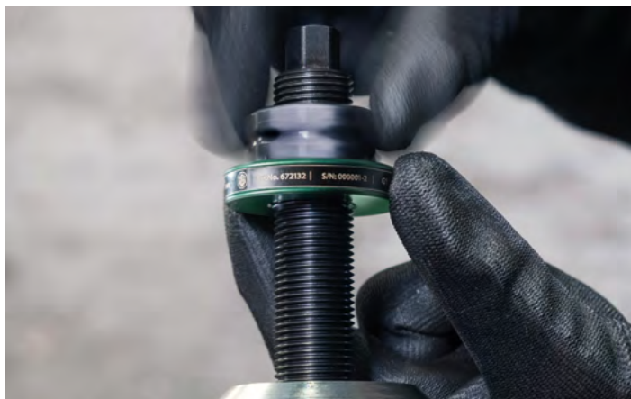
The power nut is screwed onto the spindle.
