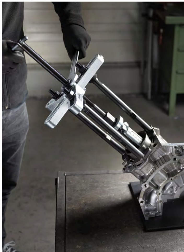
With three foot bolts on the multi traverse, you have an optimal stand during the extraction process with the cylinder bush puller 16-2.
