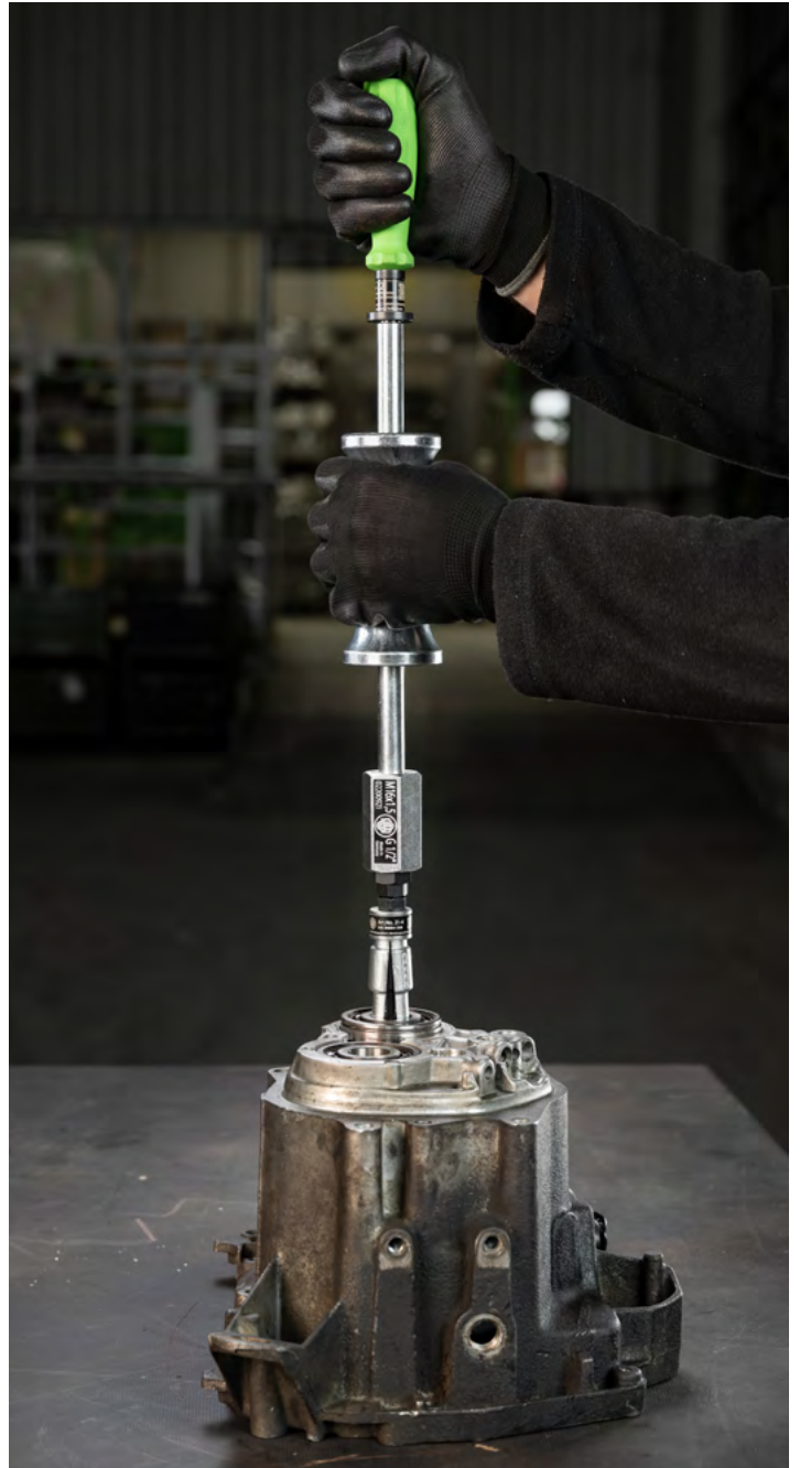
Internal extraction of a ball bearing with the 21-4 and a sliding hammer
