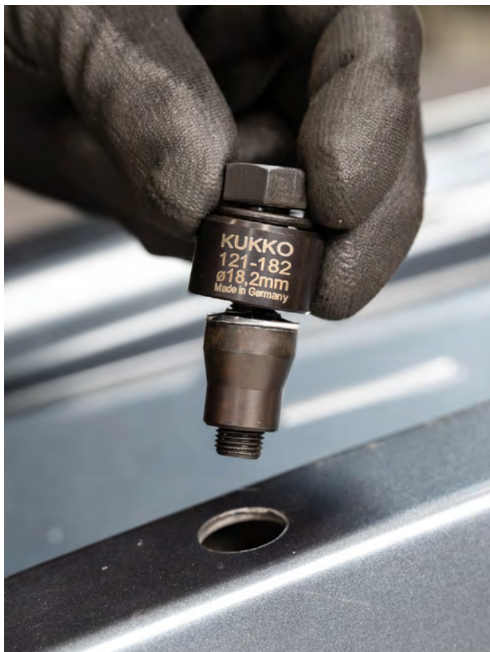
The screw punch 121-182 is inserted through the previously drilled hole.
