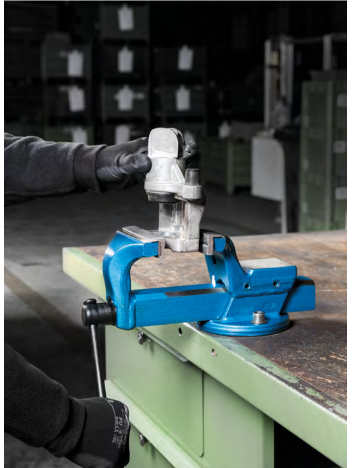
Clamping a workpiece with a vise from the 525 series.
