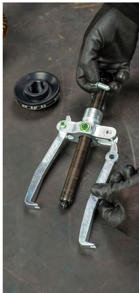
Turning the puller legs
