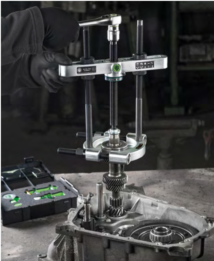
Removing a bearing from a gear shaft
