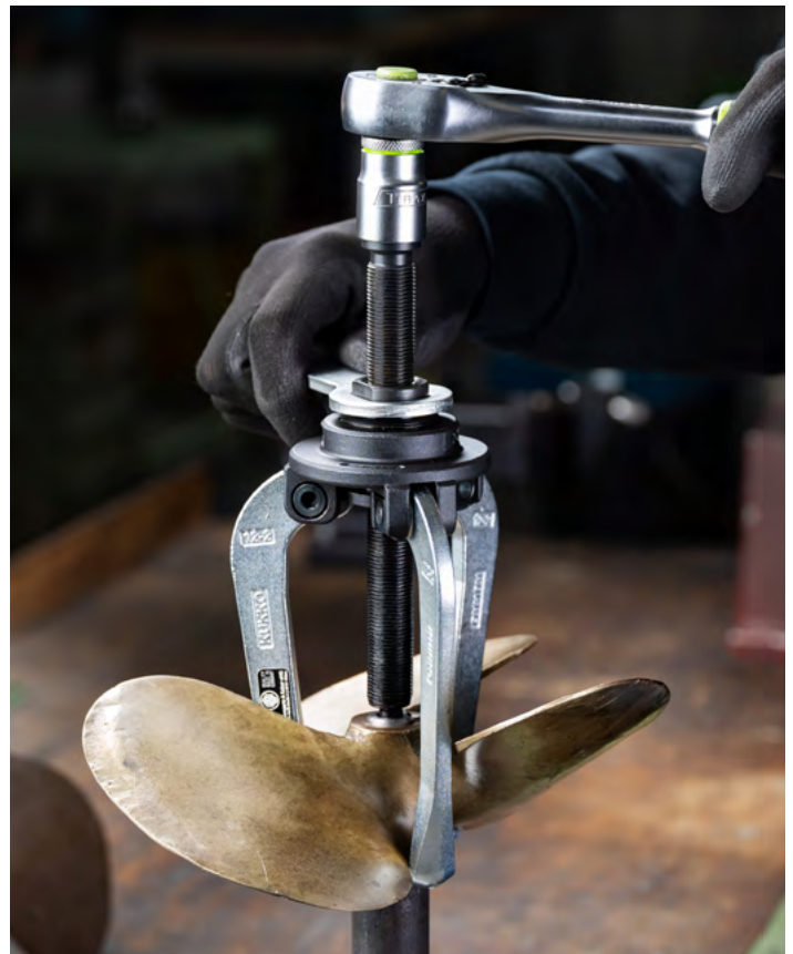
Dismantling a ship propeller with the 12-2
