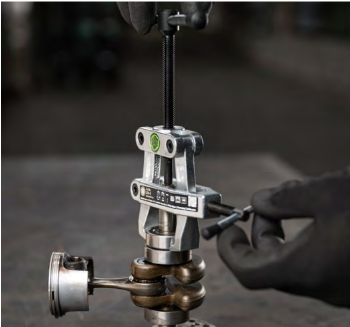
Removing a ball bearing from a crankshaft of a chainsaw with the 204-0
