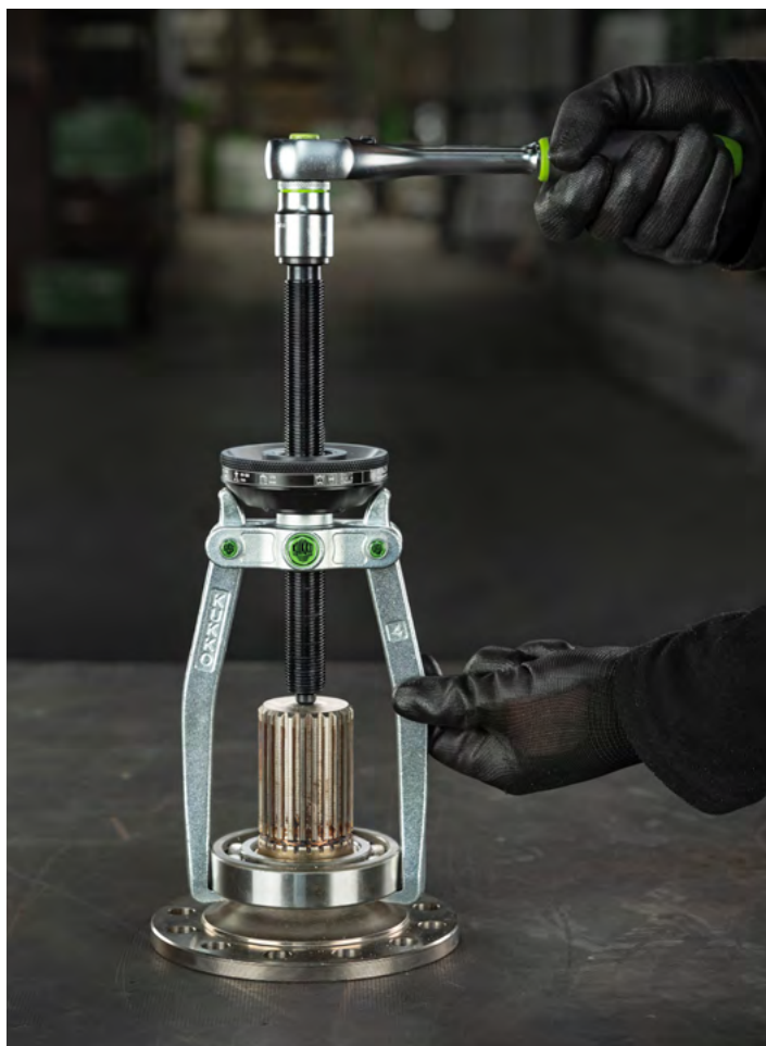
External removal of a ball bearing from a drive shaft
