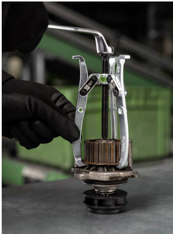
Removing a fan wheel with the 209-0.
