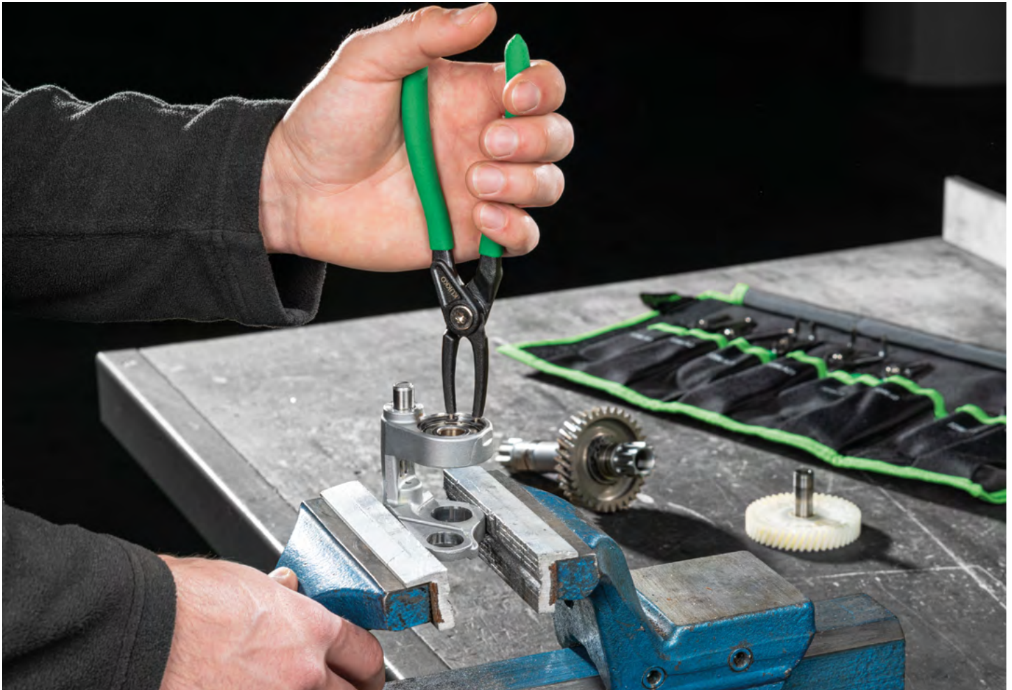
A pair of pliers from the circlip pliers set 728K-729 is used to remove a stuck circlip
