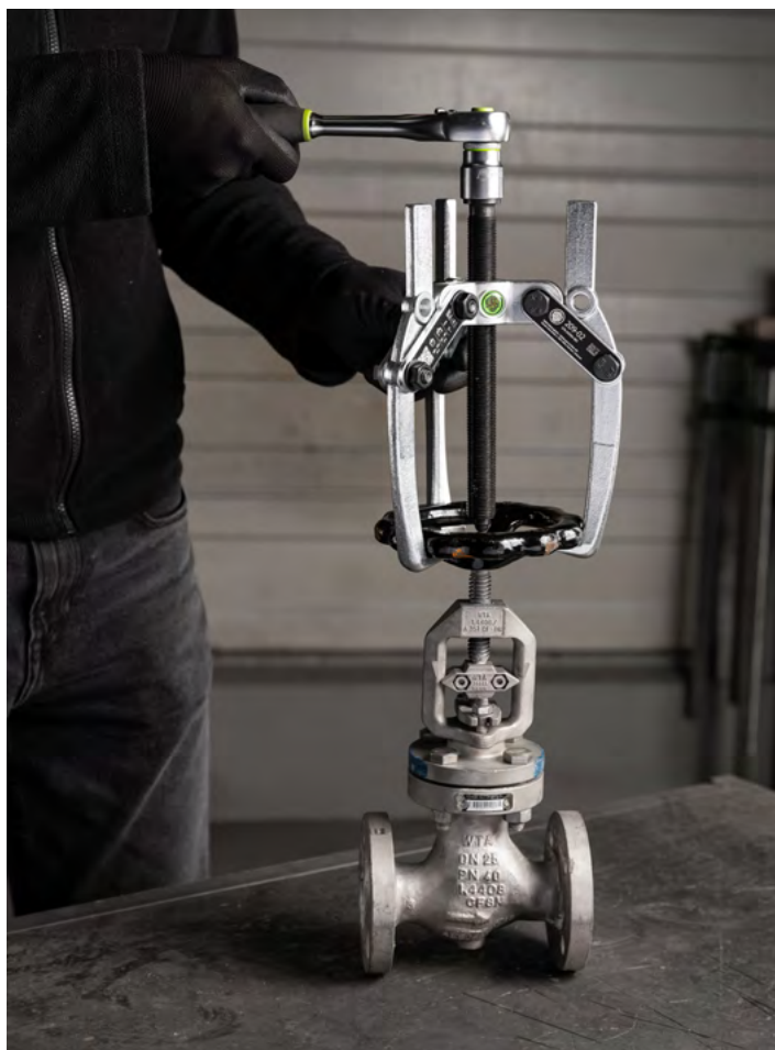
Removing the handwheel from a shut-off valve with the 209-02.
