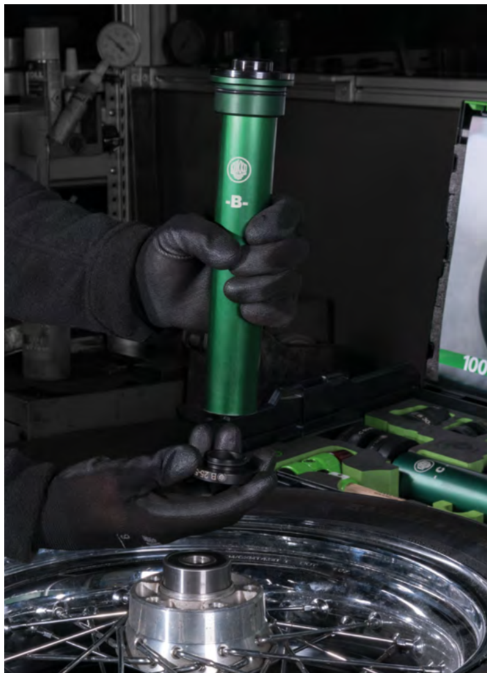
Inserting the appropriate impact ring into the impact tube when using a K-71 set
