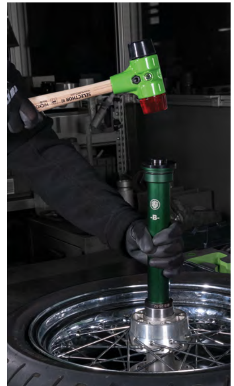
Bearing installation with the 71-L
