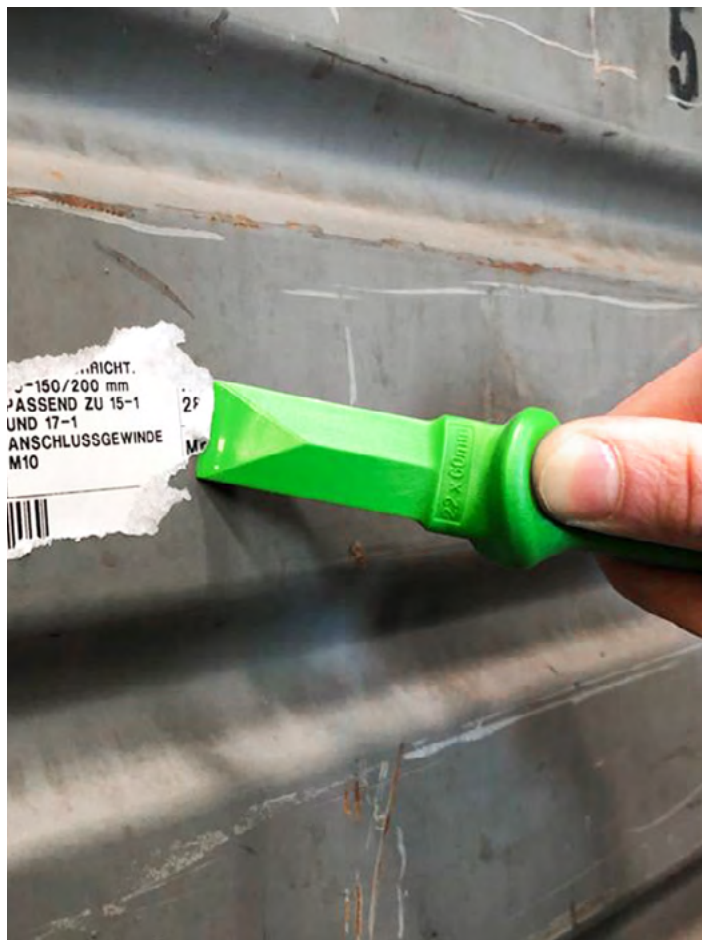
A soft scraper from the series 2200 for gently removing a product label.
